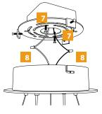
9 Reinstall canopy to backplate and retighten screws.
