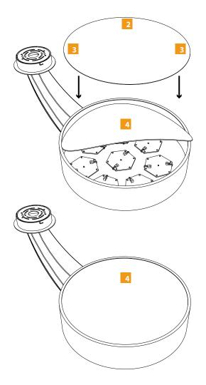
Once acrylic is in, body can hang, and acrylic should align at the base of the body.
